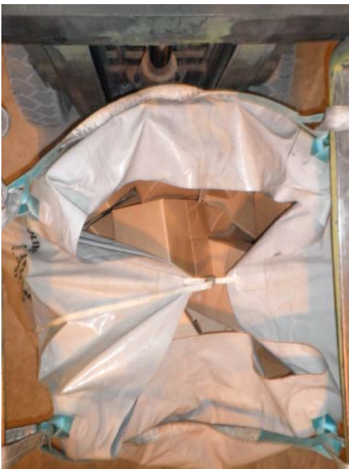
Insert strap thru clamp and pull tight
