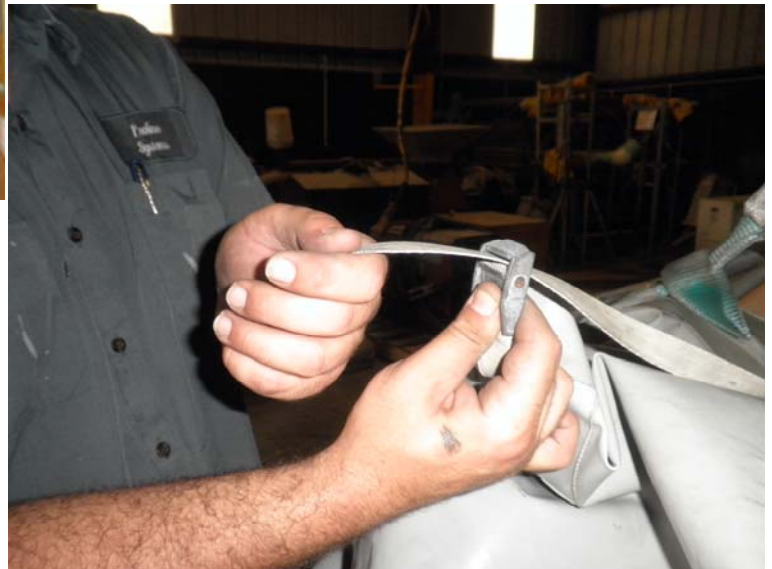
Insert strap thru clamp and pull tight
